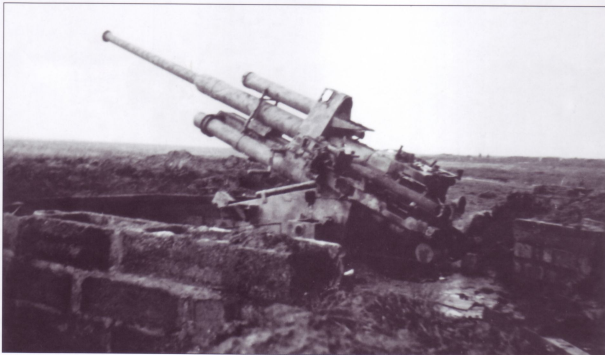
This derelict 8.8cm FlaK36 stands damaged in a city street. Note the different height of the leveling pads attached to the Kreuzlafette 36 at left and right and the sectional gun tube. This photograph also amply demonstrates that the gun could still be fired while attached to its Sd.Ah.202 limbers. Note also that the gun tube is stuck in full recoil and has four "kill rings" painted around the so-called "spring-nut", which was the part that held the sectional gun tube together.
