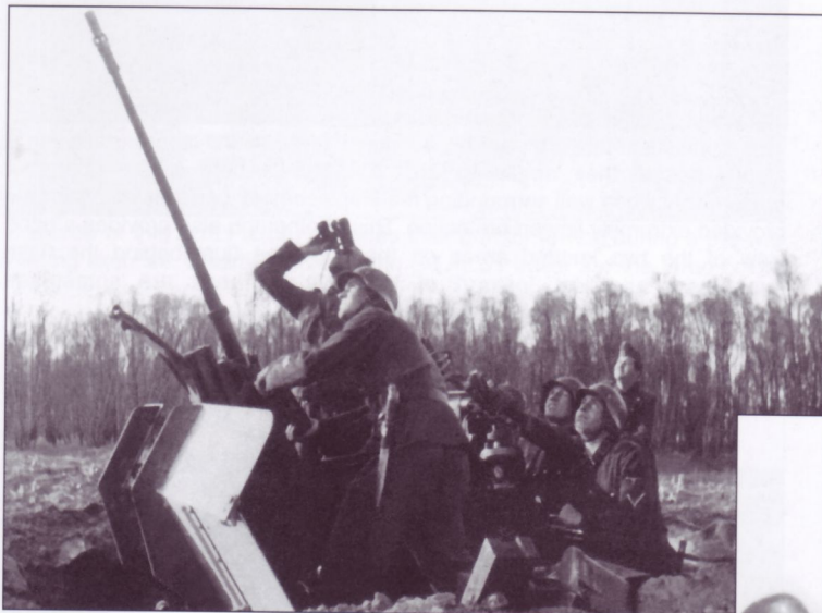
Two members of a Gebirgsjäger-Regiment (note the "Edelweiss" trade badge on the sleeve of the gunner) practice with their 2cm FlaK30. Two features of this gun are noticeable here: the unique style of muzzle flash suppressor and the centralized location of the gunner's seat. Both differed from those seen on the later 2cm FlaK38.
