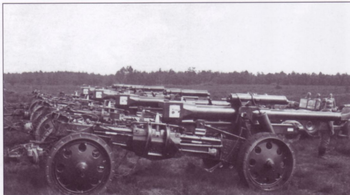
This photograph provides an excellent view of a battery of 15cm s.FH18s ready for hauling by motor vehicles. Several details of note include the position of the earth spades, as well as the location of tools and accessories on the sides of the trail legs; the brake and electrical lines that run from the tractor to the limber are also shown as is the limber itself. Note that there are also rather robust retaining chains attached to the earth spades, and that the sliding wedge breech block is in a bright natural metal color. The near piece has a sprayed "feuersicherem Buntfarbenanstrich" three-tone camouflage pattern with soft edges.
