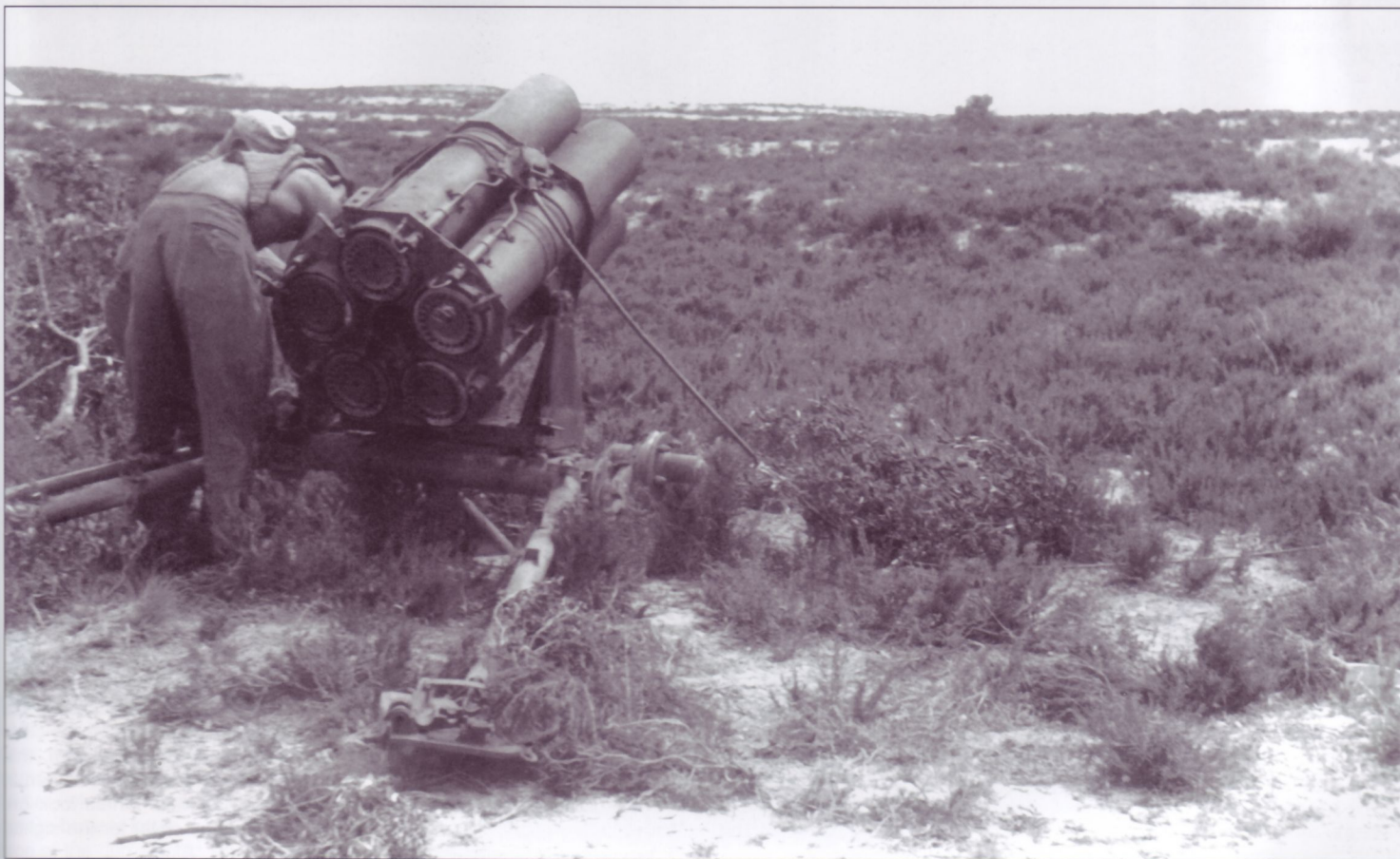
This pair of photographs depicts the crew of a 21cm NbW42 preparing their weapon for a fire mission, probably in Tunisia in early 1943. In the first photo, note the cable running from the right of the launcher; this was connected to a firing plunger that was detonated remotely in order to avoid the considerable back-blast from the rockets. The rockets themselves are in place (note their bases with venture tubes around their rims) and are held stationary by small levers. In the second photo, the bulk of the crew has moved a safe distance away as one man makes a final adjustment. Curiously, the wheels have been removed from this launcher.
