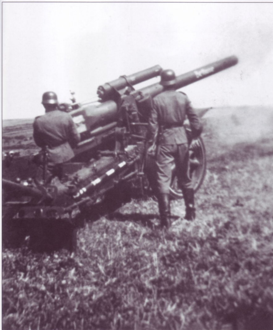
This 15cm s.FH18 sits beneath camouflage netting held up by saplings as a crewman relaxes in between fire missions. Note the gun-in-battery letter, "D", on the breech block, as well as the two hand-wheels behind the back of the crewman. The outer hand-wheel traversed the piece, while the inner hand-wheel provided for precision elevation control; the afore-mentioned auxiliary hand-crank on the trail leg provided for rough elevation.
