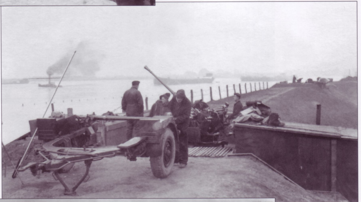
A pair of 3.7cm FlaK36s (or 37s) provides protection to a harbor somewhere in north-western Europe. The near gun is emplaced below the level of the earth sea-wall and is surrounded by a wood slat working platform; to the rear is a shelter for the crew, with a welcome heat source. Note that the Sd.Ah.52 trailer is propped up on its landing skid, providing a fine view of it in this particular configuration.
