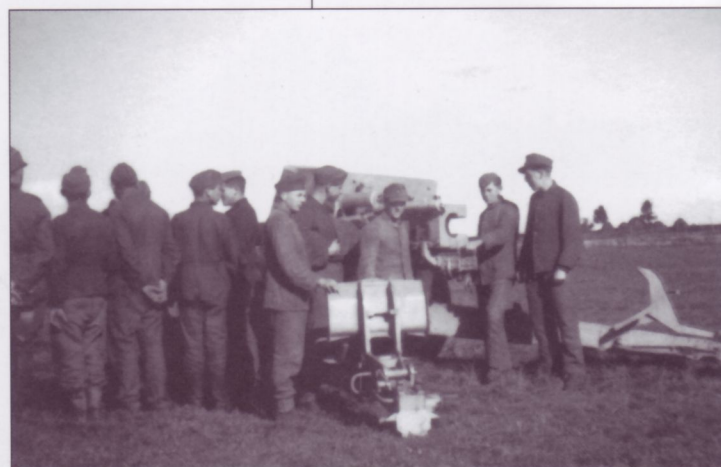
This rear view of the 8.8cm PaK43/41 shows the characteristic folding spades fitted on the split trails, a holdover from the original 10.5cm I.FH18; also clear in the photo is the gun's breech. Note that this hybrid was excessively tall and therefore much more difficult to conceal in an ambush position. Furthermore, the gun's relatively high weight made it far more difficult to displace using manpower alone.
