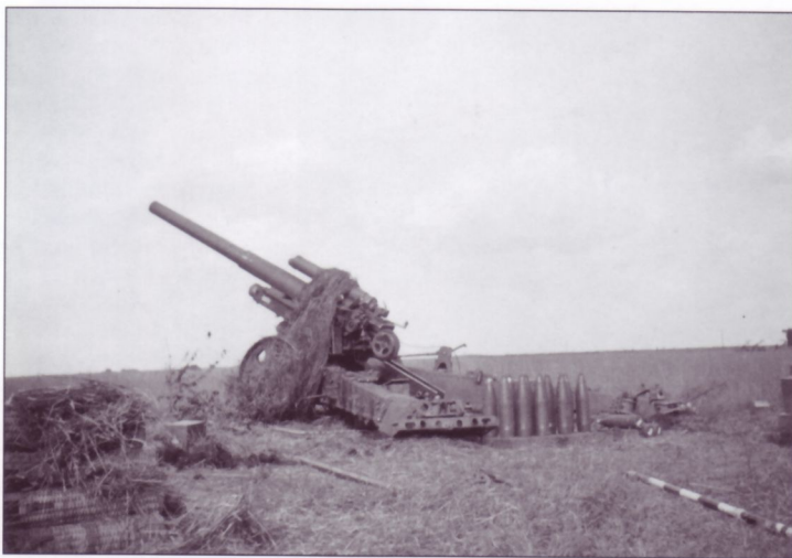
With shells arrayed ready for use, this 15cm s.FH18 awaits a fire mission. Note that the earth spades are properly dug-in at the ends of each trail leg and the striped aiming stake in the right foreground. The wicker tubes at left held powder charge increments, and an attempt has been made to conceal them with foliage, while some type of netting has been draped over the howitzer's carriage for use in distorting its outline. Also prominent is the auxiliary elevation crank on the far trail leg and the shaft that connected it to the mount.
