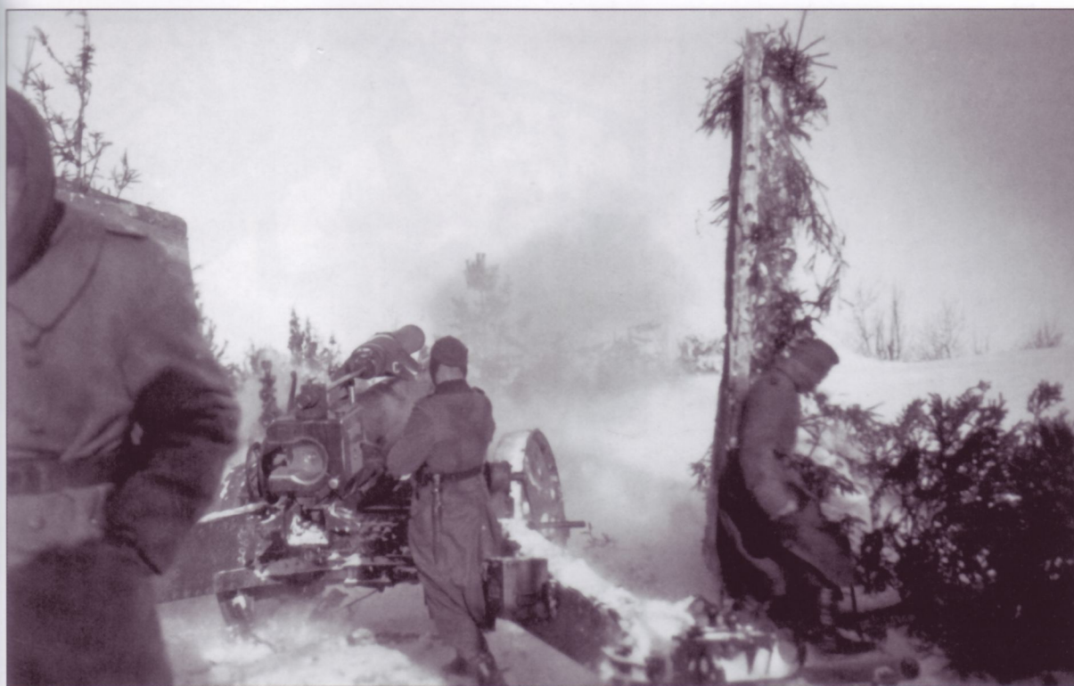
The stable-mate of the 10cm K18 was the very similar appearing 15cm s.FH18, a heavy field howitzer, seen here in full recoil. The identifying feature in this photograph is the larger opening in the breech block to accommodate the larger-diameter 15cm cartridge case. Note also how the gun has been placed next to the local vegetation for concealment.
