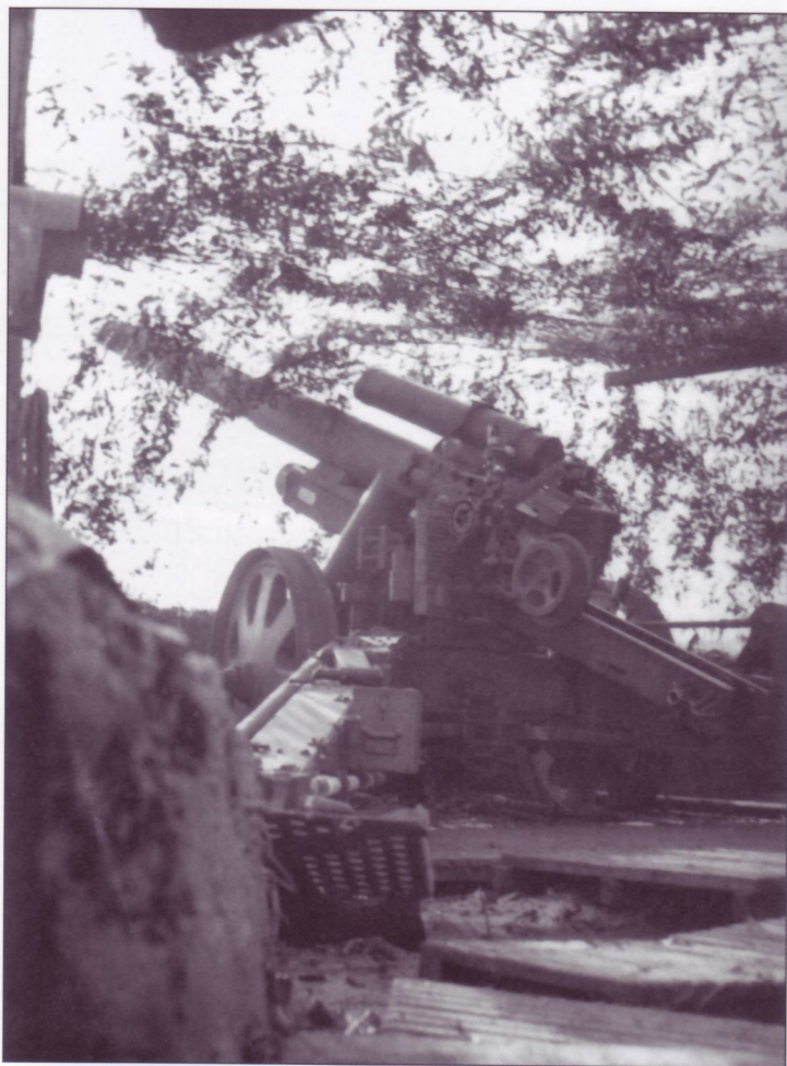
This 15cm s.FH18 is dug in beneath a rather elaborate blind constructed of timbers, netting and foliage. The crew has also laid out several sections of wood to create a work platform; these are spaced above the earth to provide drainage in what one could suppose is a relatively static position. Note again the auxiliary elevation gear crank on the right-hand side trail leg.
