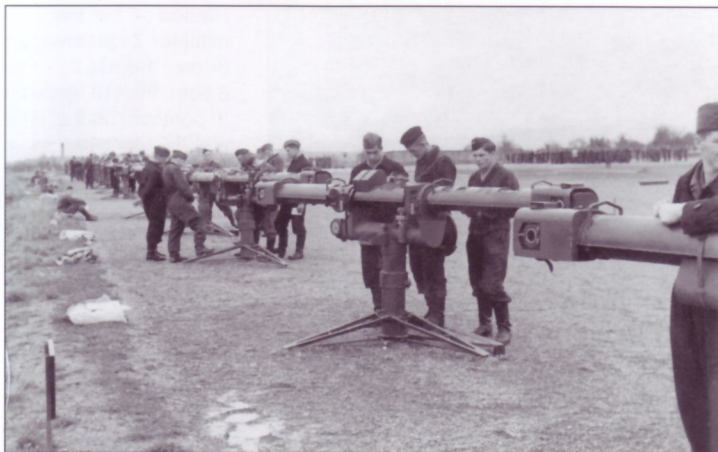
In this scene at training camp, a line of Em4 m (R) H (Raumbild-Höhenmesser, or Stereoscopic Height Gage) range-finders stretch as far as the eye can see. In the anti-aircraft role, German guns from 8.8cm in caliber, up through the 12.8cm, were centrally controlled. Data was fed into the Kommando-Hilfs-Gerät central fire control system from a variety of sources; these included visual range-finding devices (seen here), sound-ranging devices, search-lights and radar systems. Later systems mounted the rangefinder together with the central fire-control device.
