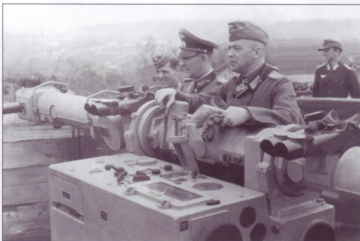
Generalleutnant Schmudt as well as several others, inspects an emplaced Kommandogerät 40, central fire-control device. This particular unit is complete with Em4 m (R) H range-finder. The entire unit could be transported on the Sd.Ah.52 trailer, which was also used to move the 2cm Flakvierling 38 and the 3.7cm FlaK36/37.
