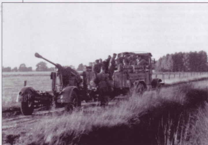
This 3.7cm FlaK18, mounted on a cruciform platform is being towed by a Büssing-NAG 3GL6 prime mover. Note also the pair of bogie units that made up the transport limber. This gun saw some service but was supplanted by the more efficient 3.7cm FlaK36 and its derivative FlaK37.
