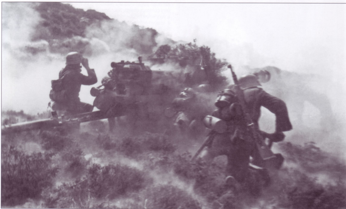
Having just fired a round, this 7.5cm PaK40 has kicked up a tell-tale cloud of dust, compromising its position. Note that one crewman is bearing down on the spade at the end of the trail legs to help steady the gun, while the commander observes the fall of shot.
