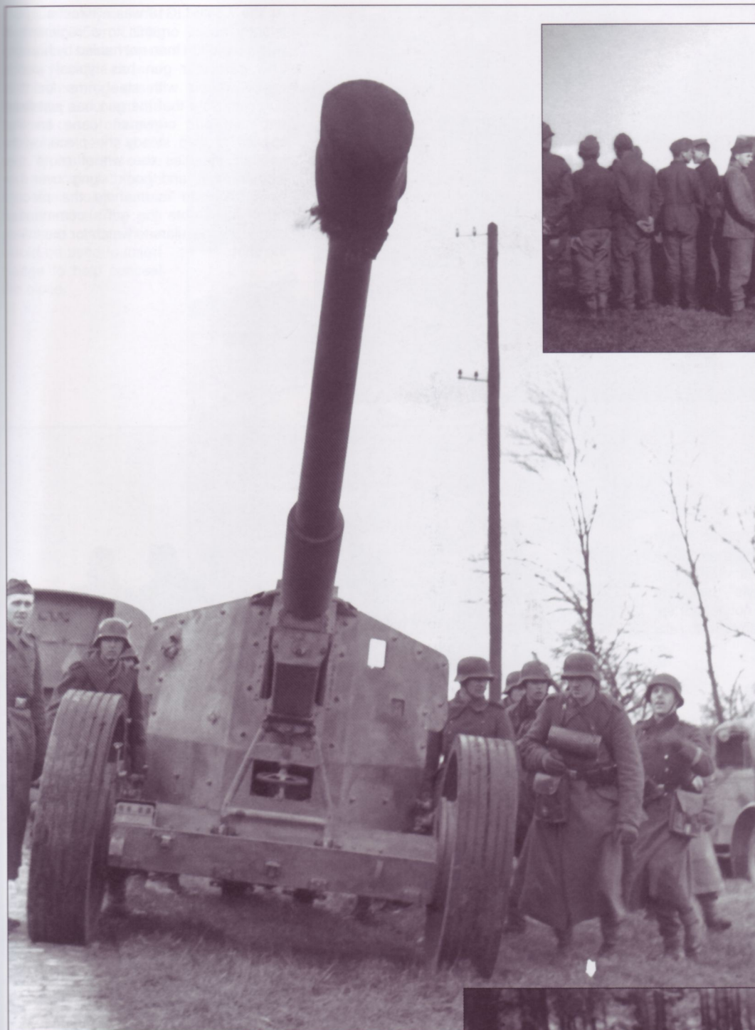
This rear view of the 8.8cm PaK43/41 shows the characteristic folding spades fitted on the split trails, a holdover from the original 10.5cm I.FH18; also clear in the photo is the gun's breech. Note that this hybrid was excessively tall and therefore much more difficult to conceal in an ambush position. Furthermore, the gun's relatively high weight made it far more difficult to displace using manpower alone.
