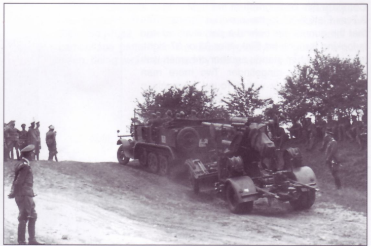
Another pre-war photograph depicts an 8.8cm FlaK18 in tow, this time by a mittlerer Zugkraftwagen 8-ton Sd.Kfz.7 with the early Kmm8 body style. Note again the Reichsheer-Wehrmacht registration numbers on the side and rear license plates, the cable reels for the fire control data transmission system on the limber, and the cover over the breech of the gun. A group of officers observe the gun's movement from under the shade of some saplings, while a Luftwaffe officer, complete with ceremonial dagger, gets a closer look at the proceedings.
