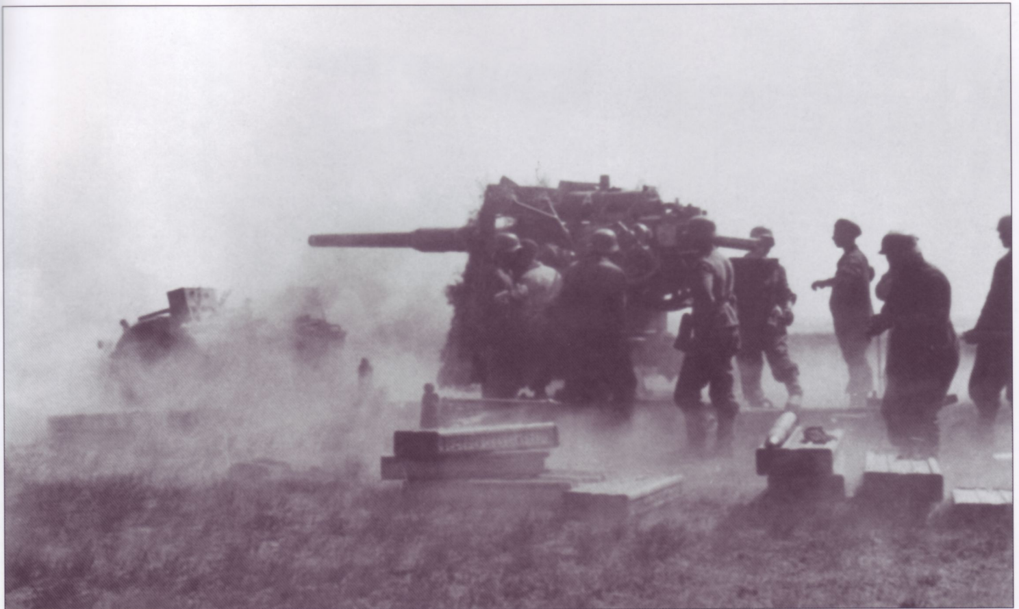
Caught in full recoil immediately after firing (note the spent case being ejected from the semi-automatic breech), this 8.8cm FlaK has raised a cloud of dust from the concussion of the projectile leaving the gun tube. Note the "A" on the pneumatic recuperator, the small shield towards the front of it, and the larger Schützschild (splinter shields) fitted to the main mount. This piece is also fitted with the sectional gun tube.
