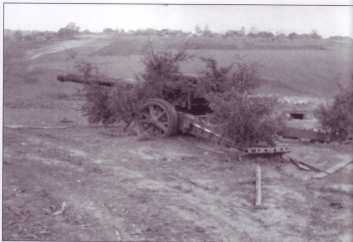
Emplaced in the open on gently rolling terrain, this 15cm s.FH18 has been partially concealed by cut evergreen tree branches. Note that the breech and muzzle have covers in place to protect against the elements and that the wheel pattern is of the less common "star" pattern.
