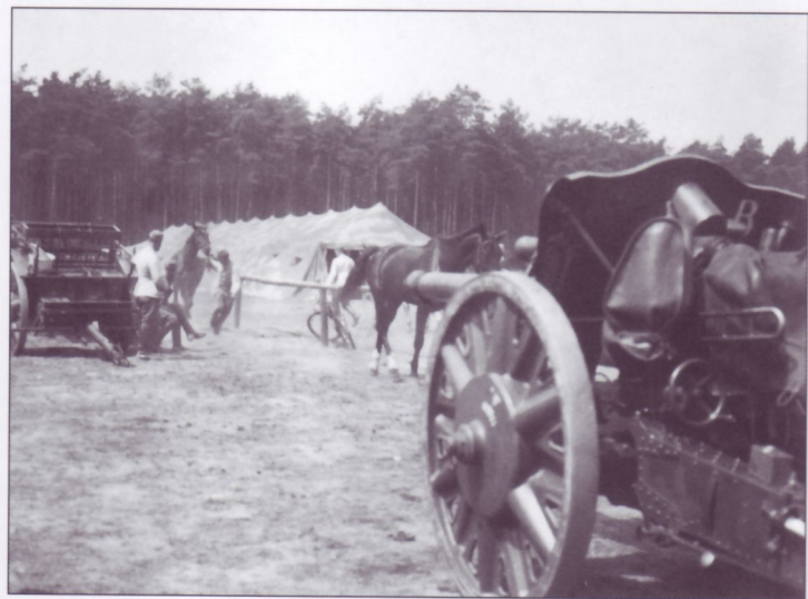
Seen in camp prior to the outbreak of hostilities (note the pre-war, three-color "feuersicherem Buntfarbenanstrich" camouflage scheme on the gun), this 10.5cm I.FH18 is apparently awaiting its turn to be attached to its limber. In the background, some crewmen ready their horses, while others look on. Visible on the gun is also the customized foul weather cover for the sights, the cover for the breech and the gun-in-battery letter, "B".
