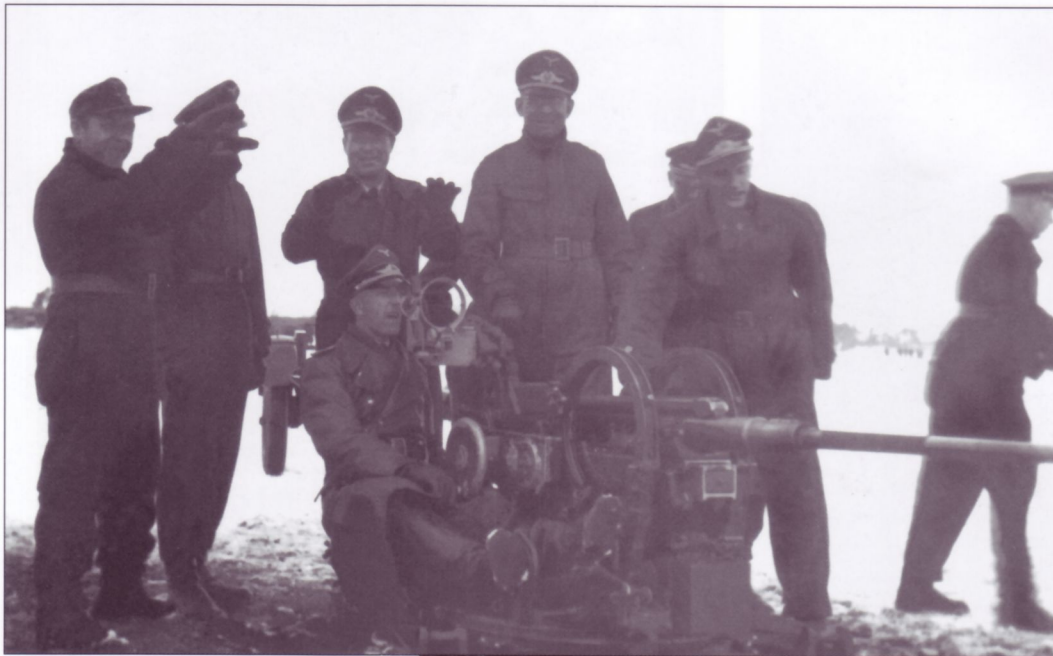
A group of Luftwaffe officers seem to be enjoying themselves as they "play" on a 2cm FlaK38. Note the characteristic circular elevation trunnion bearing assembly and the pattern of metal work on the gun tube. The gun was loaded through the circular opening on the left side of the bearing assembly, and the spent cartridge cases were ejected from the right side; sometimes a rod and net device was fitted to catch them.
