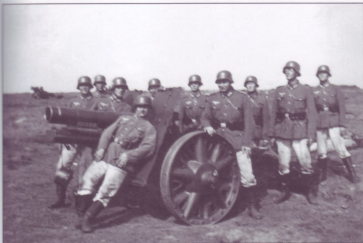
The gun crew of this 15cm s.IG33 poses with their piece during training. Note the men all wear their white fatigue trousers with their otherwise standard field uniform. The gun itself is configured for towing by horses, as can be seen by the steel-rimmed wheels; note also the muzzle cap dangling from its strap, just below the front of the gun tube.
