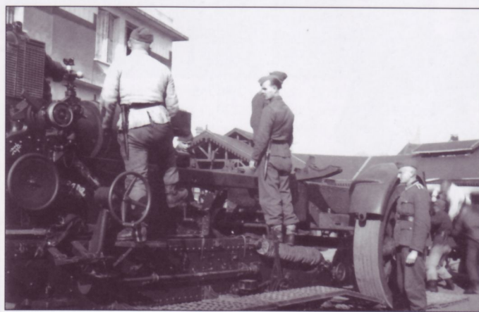
The crew of this 21cm Mrs18 is in the act of preparing to remove the gun tube for transport; note the limber pulled into position on the purpose-built ramps and the men in the background working on the piece. The limber has framework and a clamp system to secure the gun tube, which also has a separate and smaller limber (not seen here) for use in attaching the entire assembly to a tractor.
