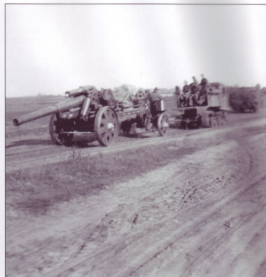
As Germany's armed forces swept deeper and deeper into the vastness of the Soviet Union, its mobility became compromised by a number of factors. So, when opportunity arose, units would become self-mechanized using captured Red Army equipment. This is a Stalingrad Tractor Factory-produced STZ-5, which is seen here hauling a 15cm s.FH18, probably from a formerly horse-drawn Infanterie-Division's organic Artillerie-Regiment.
