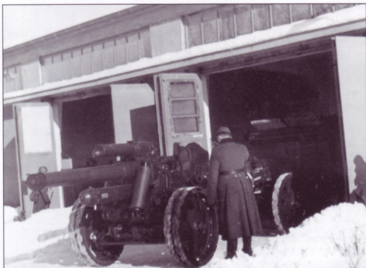
In this winter scene, a 15cm s.FH18 is being pulled into (or out of) its storage structure, which was typical of a unit's home base. The piece is immaculately maintained; the gun tube is retracted for travel and has its muzzle and breech covers in place for protection against the elements.
