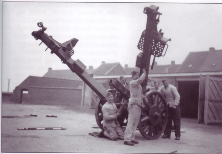
In another (rather untypical) maintenance scene, the crew of this 10.5cm I.FH18 have turned their howitzer "on its nose" in order to more conveniently work on the lower part of the carriage or mount. These crewmen also wear the white M1933 work uniform and are also just outside the garages that were used to store their pieces when not in use. At left, the striped aiming stakes have been removed and are on the ground; note also the breech cover on the recoil slide.
