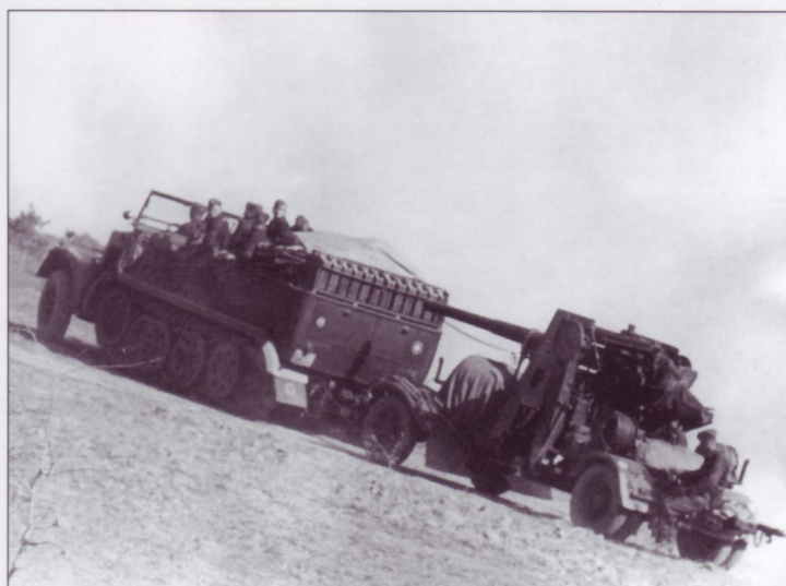
A mittlerer Zugkraftwagen 8-ton Sd.Kfz.7 rests while hauling an 8.8cm FlaK18; note the position of the brake-man on the rear section of the Sd.Ah.201 limber. Both gun and tractor are finished in overall Dunkelgrau RAL7021, with white-painted edges on the rear of the tractor and the limber unit; this was done to aid in night driving. The tractor has the insignia of the Hermann Göring Division on the right, and the insignia of 7.Batterie, II.Abteilung, Flak-Regiment "Hermann Göring" (a white disk with a tick mark at the 7 O'Clock position), at left.
