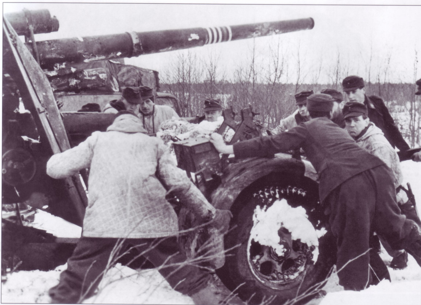
The crew of this 8.8cm FlaK36 or 37 struggle to mount one of the Sd.Ah.202 limber sections to the Kreuzlafette 36 (cruciform mount), working in the snow. Note the "kill rings" on the mono-block gun tube and the empty rack mounted on the limber that held the fire-control data transmission cable reel. The crewmember with his back to the camera wears the unique Luftwaffe-issue quilted parka with the diamond thread pattern.
