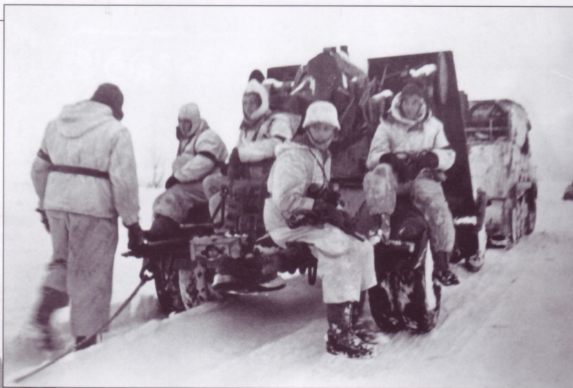
A mittlerer Zugkraftwagen 8-ton Sd.Kfz.7 pulls an 8.8cm FlaK18 through the Russian snows. The gun is identified as a FlaK18 by the configuration of the Sd.Ah.201 limbers, the round leveling pads of the Kreuzlafette 18 (cruciform mount) and the forward-pointing gun tube while in travel mode. The mount is fitted with a Schützschild (splinter shield), while the gun's breech unit is protected from the elements by a specially-fitted cover.
