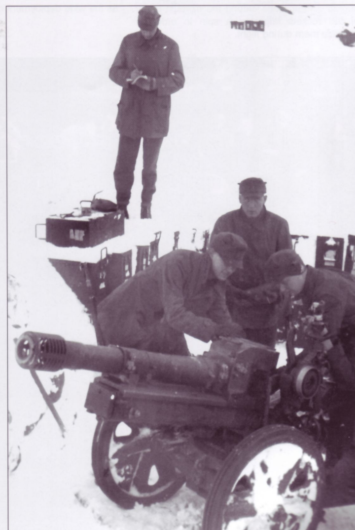
This frontal view of the 7.5cm GebG36 shows just how compact and austere a piece it really was. Note the small-diameter pressed wheel hubs with solid rubber tires, the gun-sight and the slotted muzzle brake. The gun has been dug in to a snow bank, with a parapet lined with ammunition boxes.
