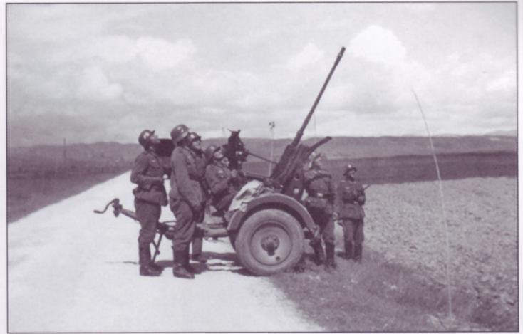
It would appear that this Heer crew (Army; note the breast eagles over their right pockets) have set up their 2cm FlaK30 in hasty fashion to engage an aerial "target of opportunity". Note the landing skid seen between the legs of the two men at left, which when extended provided some measure of stability when the gun was still on its trailer. When time would permit, the gun would be removed from the trailer, emplaced and properly leveled using pads located on the gun platform.
