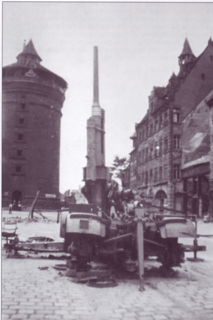
This derelict 8.8cm FlaK36 stands damaged in a city street. Note the different height of the leveling pads attached to the Kreuzlafette 36 at left and right and the sectional gun tube. This photograph also amply demonstrates that the gun could still be fired while attached to its Sd.Ah.202 limbers. Note also that the gun tube is stuck in full recoil and has four "kill rings" painted around the so-called "spring-nut", which was the part that held the sectional gun tube together.
