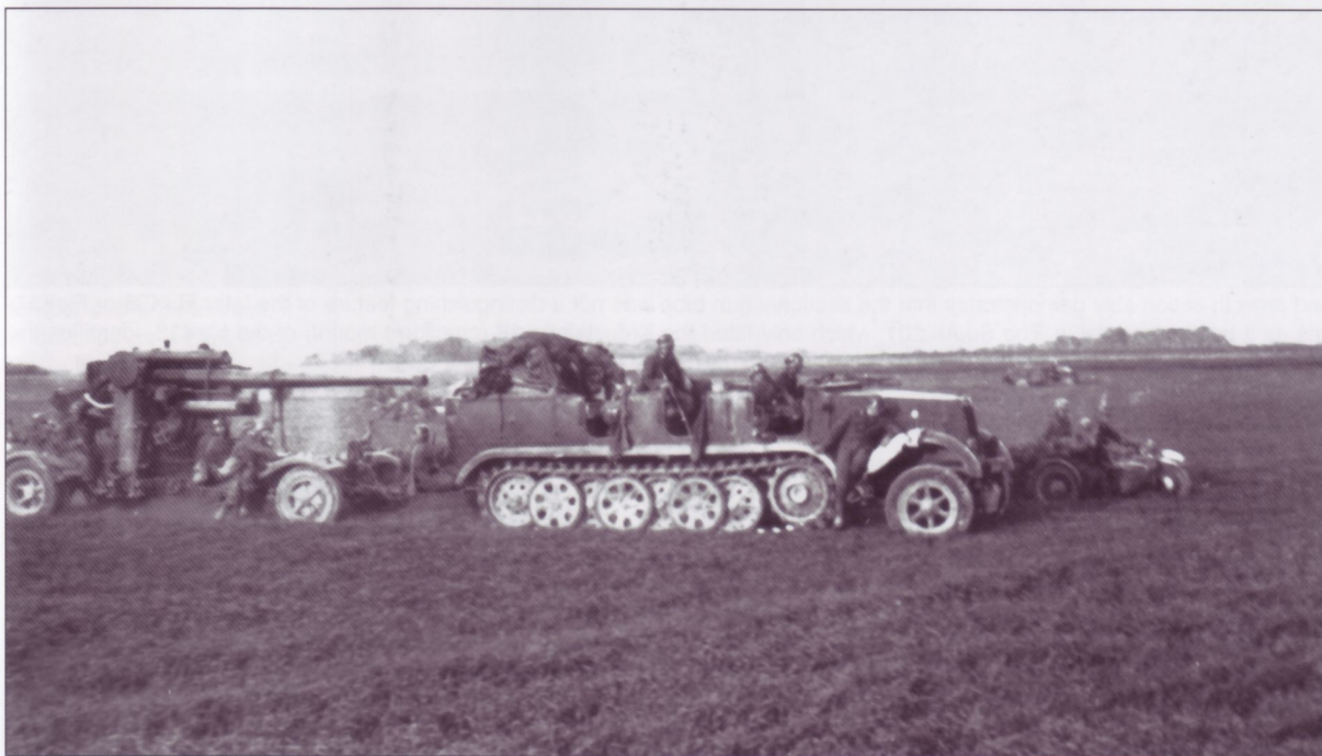
This 8.8cm FlaK18 is being towed by its standard tractor, the mittlere Zugkraftwagen 8-ton Sd.Kfz.7. The tractor has the later KMm11 body style, while the FlaK18's gun tube is pointing forward. The latter feature, the round leveling pads of the Kreuzlafette 18 (cruciform platform) and the Sd.Ah.201 limber units clearly identify the specific gun type.
