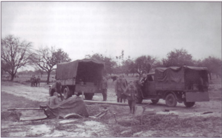
Members of a Heer (Army) gun crew approach their dug-in and canvas covered 2cm FlaK30. It is mounted on its Sd.Ah.51 trailer and can be attached to its tractor at a moments notice. The light truck behind it is unidentified, while the larger truck is a 3-ton Opel or Ford.
