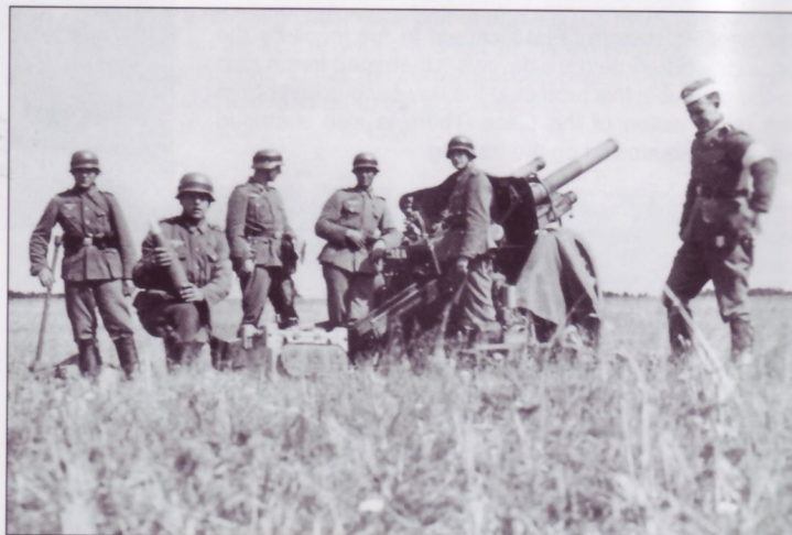
Seen here during training maneuvers (note the white band on the umpire's cap at right and the darker bands on the helmets of the gun crew), this 10.5cm I.FH18 crew prepares for a fire mission. Note from left to right, the crewman with the ramming staff, and the man kneeling, holding a projectile. The 10.5cm I.FH18 was loaded with a separate projectile, adjustable powder increments and a primed cartridge case; the latter item was also used to completely seal the piece's breech.
