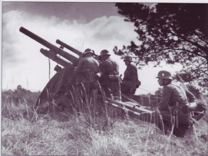
A German Heer (Army) crew prepares to fire their 10.5cm I.FH18, probably during a training exercise. It would appear from this and other photographs that the crews commonly hung a tarp on the gun's wheels, possibly to conceal the shape or to prevent any reflections of the steel hubs from being seen at a distance. Note also how the canvas cap that covered the muzzle during travel is hanging from a strap below the elevated gun tube.
