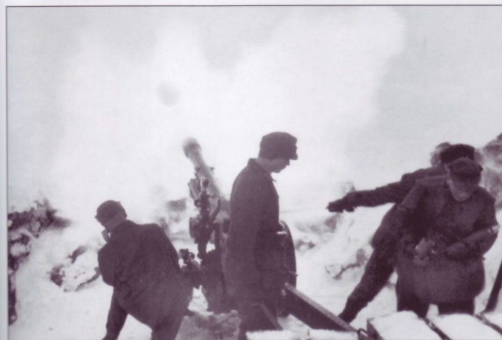
Germany's Gebirgsjäger-Divisionen (mountain divisions) also fielded their own specially-designed organic artillery, in this case the 7.5cm Gebirgsgeschütz 36. The gun has just fired; note the muzzle flash and the crewman's hand pulling the firing lanyard. The gun could be broken down into several loads for transport by mules, the Sd.Kfz.2 Kettenkraftrad, or by manpower.
