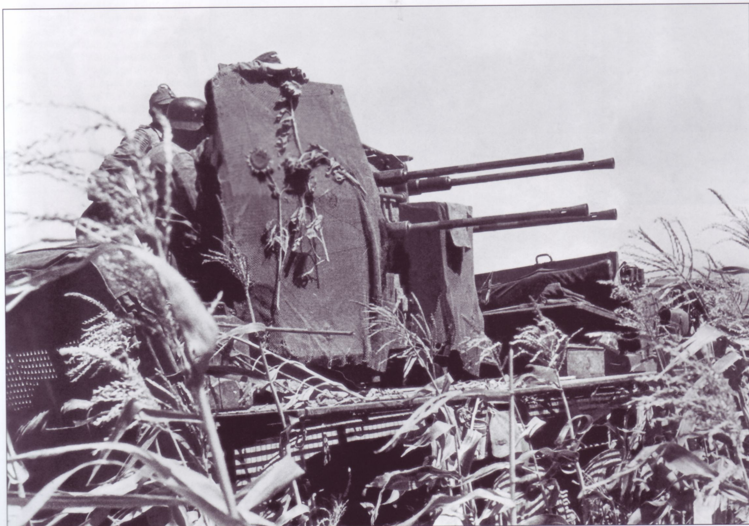
The 2cm Flakvierling 38 was mounted on several different vehicles as self-propelled units. Here the gun is seen on a mittlerer Zugkraftwagen 8-ton Sd.Kfz.7/1 half-track. The vehicle itself is well camouflaged by the standing grain, while the gun also has the remains of some sunflowers on the shield, presumably originally fitted to break up its outlines.
