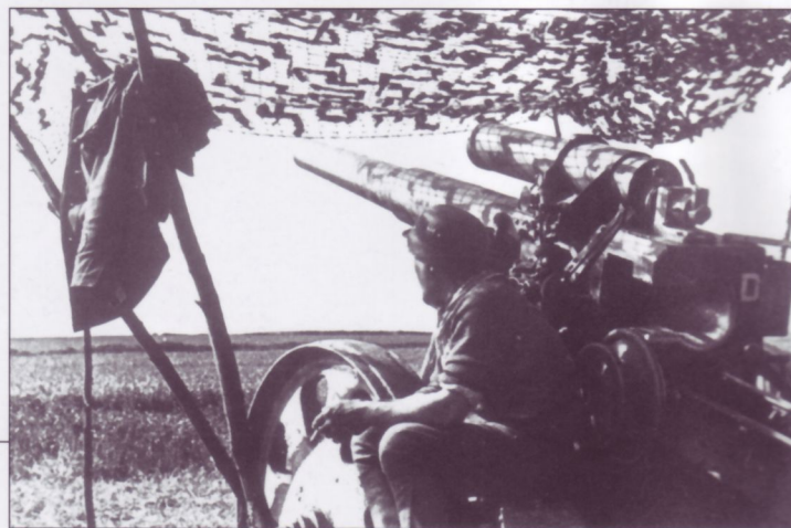
The photographer has caught this 15cm s.FH18 in full recoil, but unfortunately the name on the gun tube is blurred. Note that the earth spades are not fully dug in, suggesting that the gun was hastily set up or, that this is a training scene. Note the striped aiming stake secured to the near trail leg.
