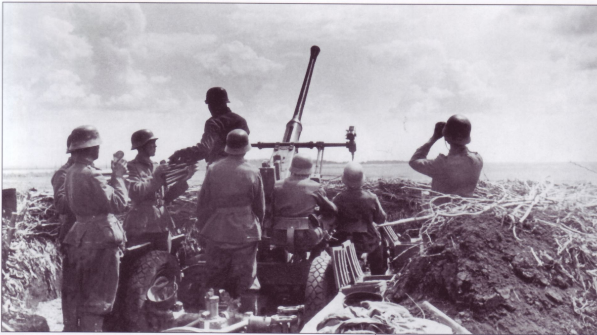
A German gun crew serves this dug-in 4cm FlaK28 (Bofors). Note the ammunition handlers lined up with four-round clips of ammunition to feed this hungry gun. This gun was externally very similar to its un-licensed Soviet counterpart, the 37mm Anti-Aircraft Gun Model 1939, which in German service was designated 3.7cm FlaK M.39a(r). From this angle, the mounting system for the gunner's sights most resembles that seen on the Bofors gun.
