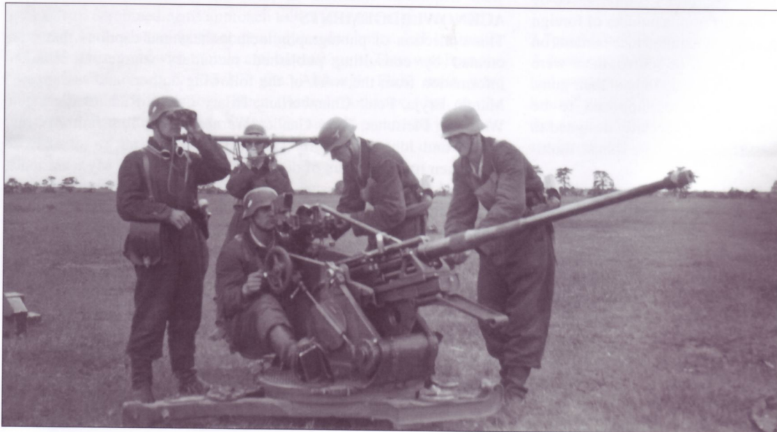
The crew of this 2cm FlaK30 prepares their gun for towing during a pre-war training exercise. Clearly visible on the Sd.Ah.51 trailer are the three colors of the "feuersicherem Buntfarbenanstrich" camouflage scheme. In this case, the colors are sprayed on creating a soft edge between them.
