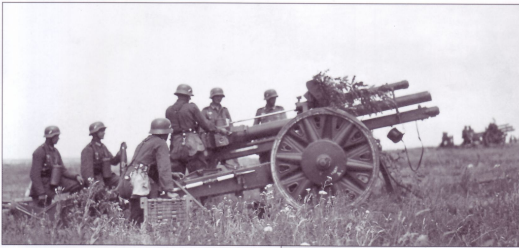
This 10.5cm I.FH18 has been caught at the moment of full recoil by the photographer; note how the shock of the weapon being fired has caused the canvas gun tube cover to "dance" on its attachment strap. As seen in a previous photograph, many of the crewmen wear their gas mask canisters hung over the front of their bodies. Note the striped aiming stake on the trail legs and the unusual configuration of the wicker ammunition (or fuse) container seen behind the kneeling man in the foreground.
