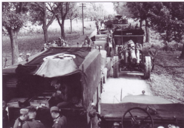
A variety of military vehicles, along with those of an artillery unit, clogs a road, probably during the French Campaign of 1940. Among them is a tractor hauling a 15cm s.FH18; note the gun-in-battery letter, "B" painted on both elevation counter-balance cylinders, either side of the gun tube. The lorry at left is draped with a typical aerial recognition device, a Nazi Flag.
