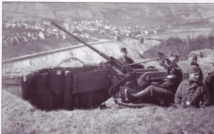
This well-emplaced 2cm FlaK30 guards a river crossing, probably during pre-war exercises; note the "feuersicherem Buntfarbenanstrich" three-tone system of Nr.17 Erdgelb-matt, Nr.28 Grün-matt and Nr.18 Braun-matt, seen here in a hard-edge pattern. This scheme was officially dispensed with in July of 1937.
