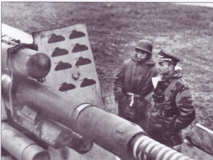
A Luftwaffe officer and one of his men stand idly next to their rather successful 8.8cm FlaK gun. There are silhouettes of eight destroyed enemy tanks on the Schützschild (splinter shield) and many more "kill rings" on the sectional gun tube. The two cylinders situated side-by-side below the gun tube housed counter-balance springs, while the cylinders arranged horizontally above and below the gun tube were part of the recoil system.
