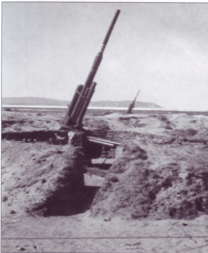
A pair of well-emplaced 8.8cm FlaK37s sit idly with their gun tubes silently pointing skywards. Note the shape of the covered Folgezeigeeempfänger (directional indicator with dials) on the near piece, which identifies the model type. The near gun has the sectional gun tube, complete with four "kill rings" just forward of the "spring-nut", which was the device that held the gun tube's component parts together.
