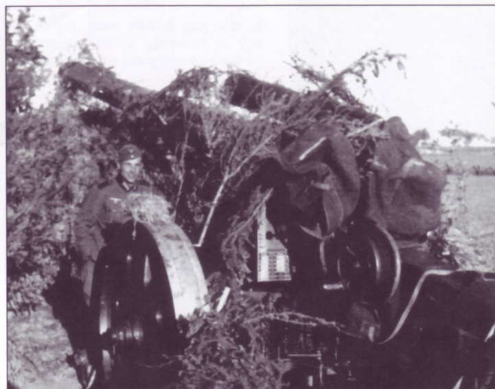
A crewman lurks behind the wheels of this well-hidden 15cm s.FH18, probably during a training session. Prominent in this photo are the covers for the breech block, the twin superimposed traverse and elevation hand-wheels and a range table placard.
