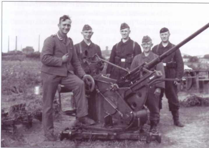
A somewhat jolly Luftwaffe Flak crew poses with their 2cm FlaK30. This crisp view affords a look at other details of the gun, notably the hooked parts of the platform that engaged the Sd.Ah.51 trailer when the piece was in transport mode. Note also the word "braun" painted in white on the gun cradle; this denoted the type of fluid used to fill the recoil mechanism.
